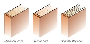
Shadcore and ENcore have a high density solid chipboard core giving consistent performance and durability.
